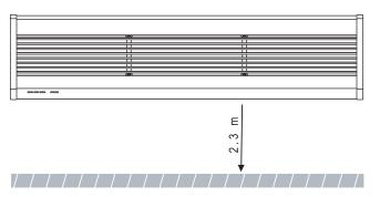
**D-** When the entrance is wider than the unit, it is recommended to install two or more units in parallel. In this case, provide 40-20mm gaps between the units.
